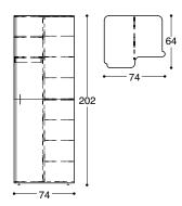
Dimensions of the aluminium cupboard: height 202, width 74, depth 64 cm
